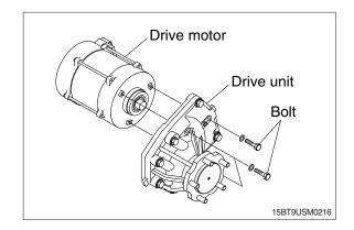
④ Loosen seven mounting bolts on the truck frame and carefully take out the drive unit.
